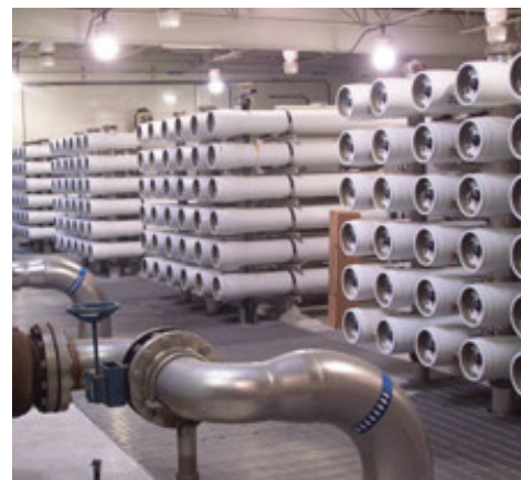
Reverse osmosis, which forces water through semipermeable membranes to remove salt, is the dominant technology used today in desalination.
